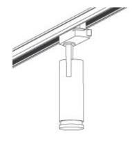
Step 2 Insert the T700.HX into the track channel, ensuring the track base tabs are in the open position and that the direction of the T700.HX is correct. This is dependant on where the contact points are in the track.
