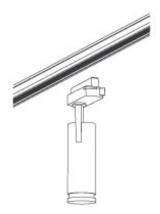
**Step 1** Align the track connector with the track.
