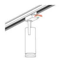
**Step 3**Push the locking tabs into the track base to secure the fitting.
