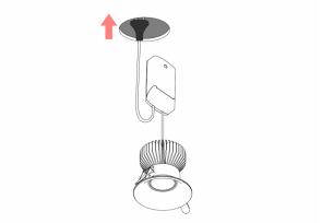
Step 2 Plug the driver into a mounted general power outlet (GPO) in the ceiling.
